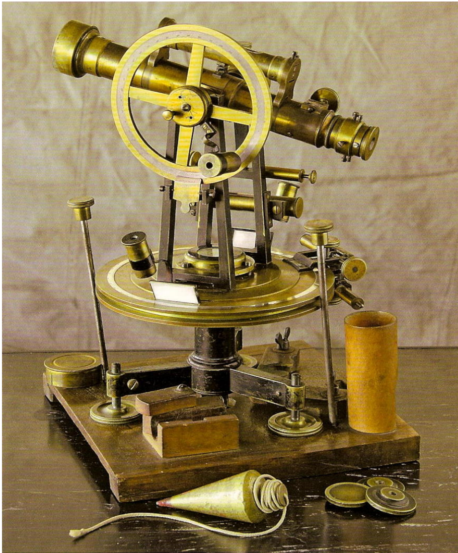
Repetition theodolite (ø 5 in.); 1865 520 Frs
